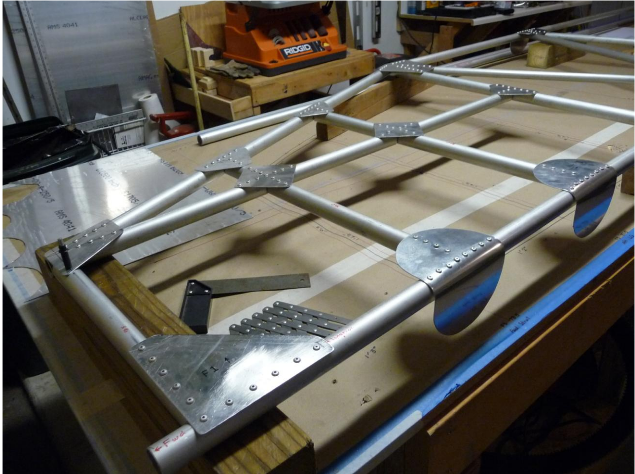
Right side forward fuselage structure showing tube and gusset construction.
