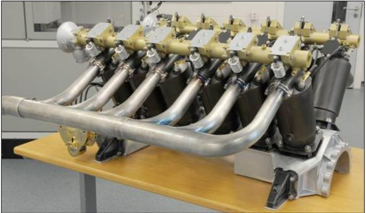
The replica Rolls-Royce Falcon engine – 95% plastic
