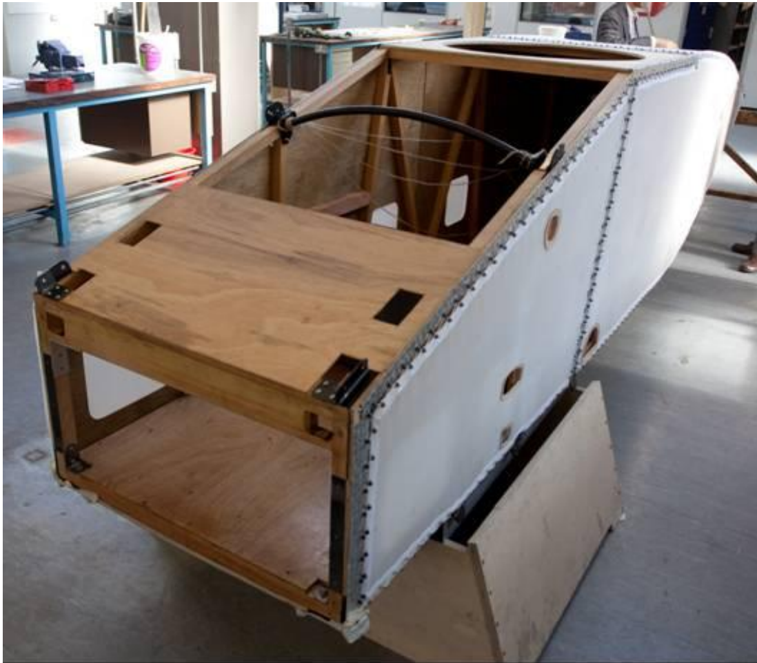
Front of fuselage after completion of fabric covering.
