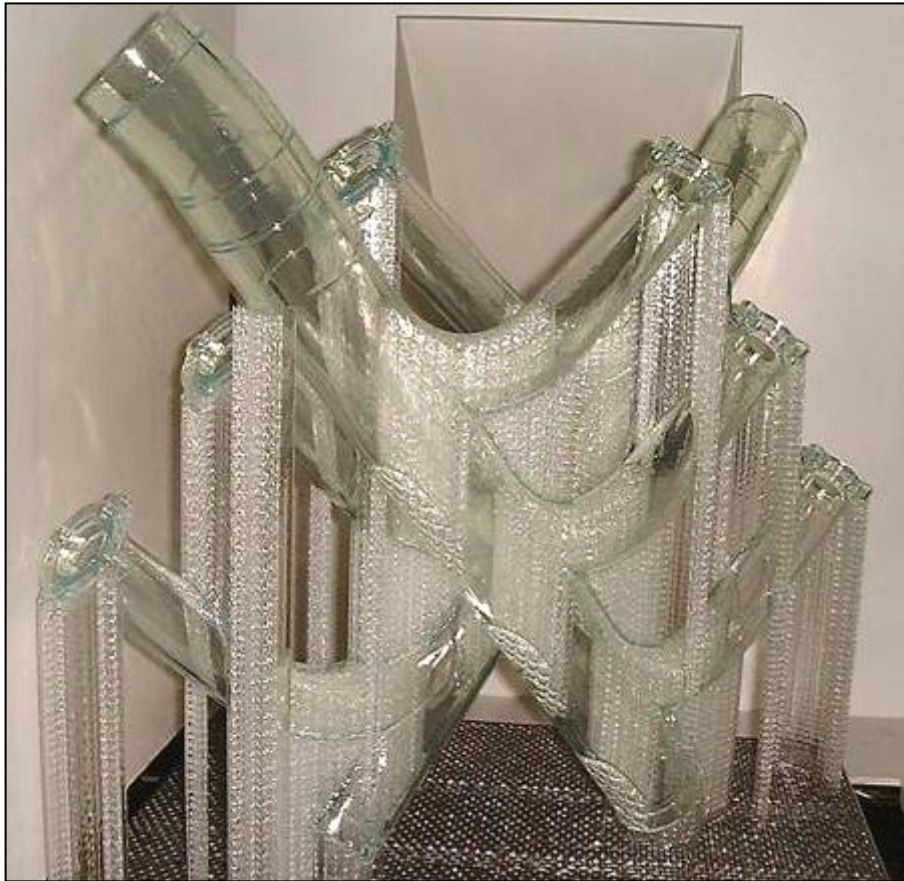
The Exhaust manifold just after completion on the Stereo Lithography printer.
