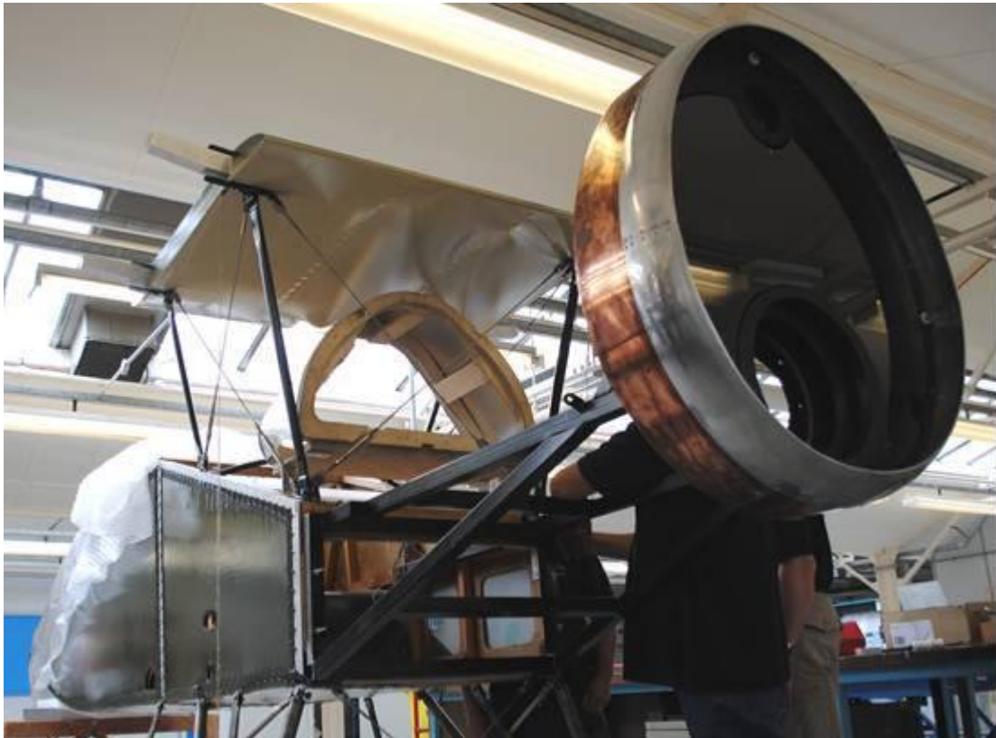
Trial fit of front end showing engine and radiator mount, dummy fuel tank and radiator.
