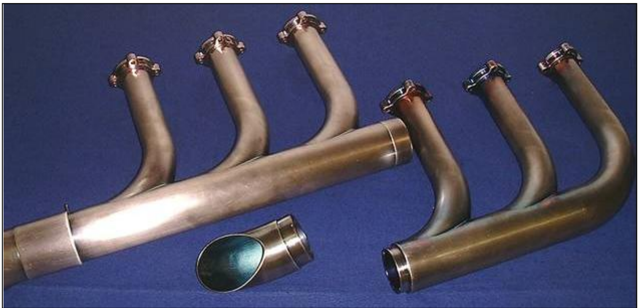
The finished exhaust manifold following metal coating
