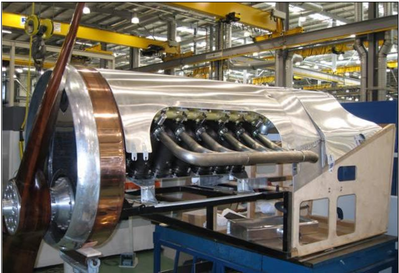
Manufacture of the front end in progress on a mock up of the fuselage.
