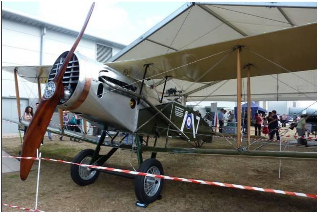
The finished article on display at the Rolls-Royce Families Day. Detail included a rotating propeller, moveable radiator slats and control surfaces.
