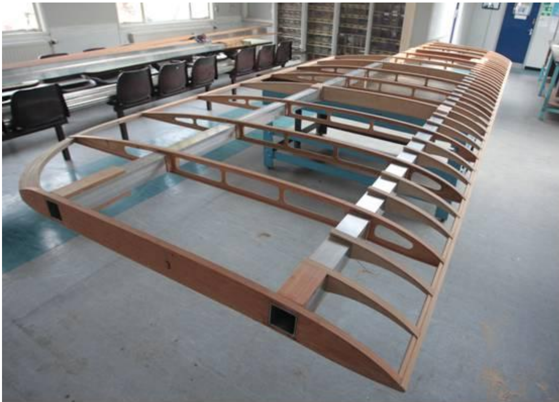
Lower wing viewed from inner end showing the aluminium main spars.
