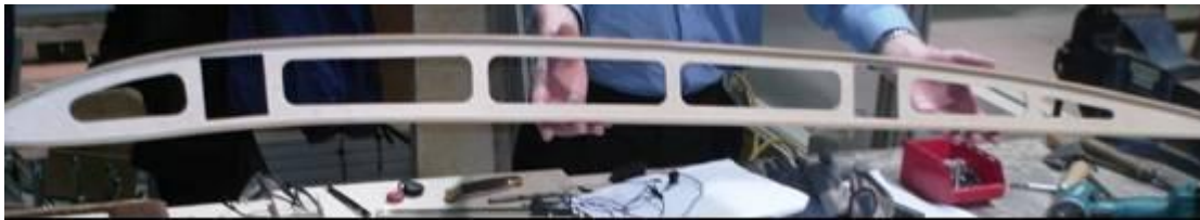
Main wing rib showing simplified construction being made from 3 pieces compared to approximately 16 pieces on original design.
