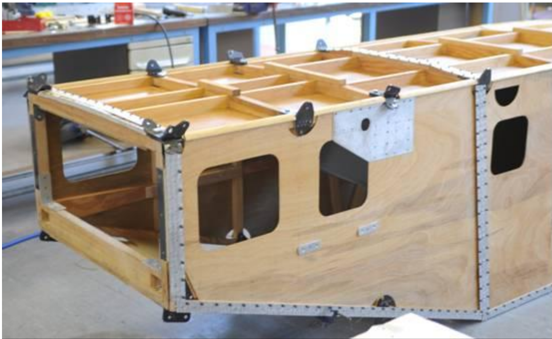
View of underside of fuselage front end showing metalwork for mounting of wings and undercarriage and lacing strips for attachment of the fabric covering. Metal brackets were similar to original design.
