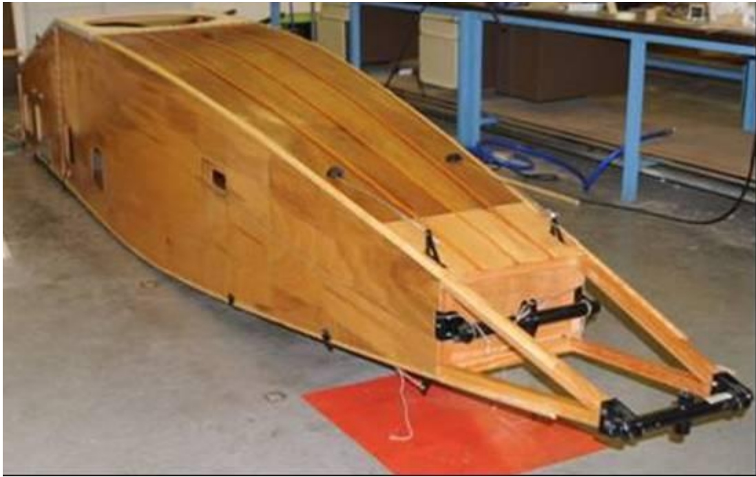
Finished fuselage prior to fabric covering.
