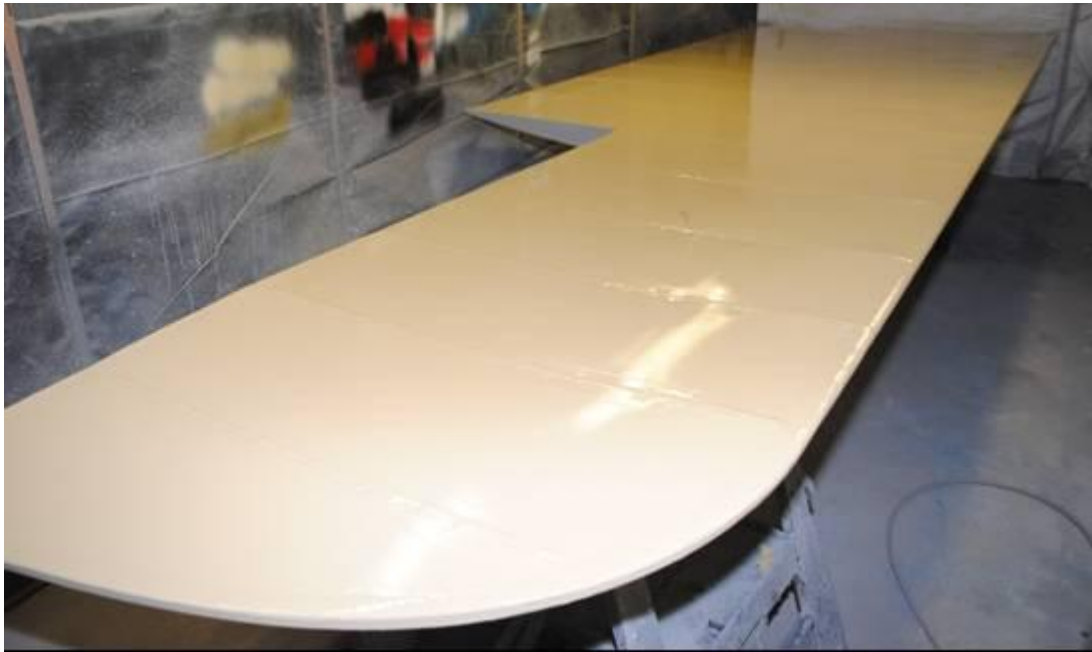
Underside of lower wing after covering and painting.
