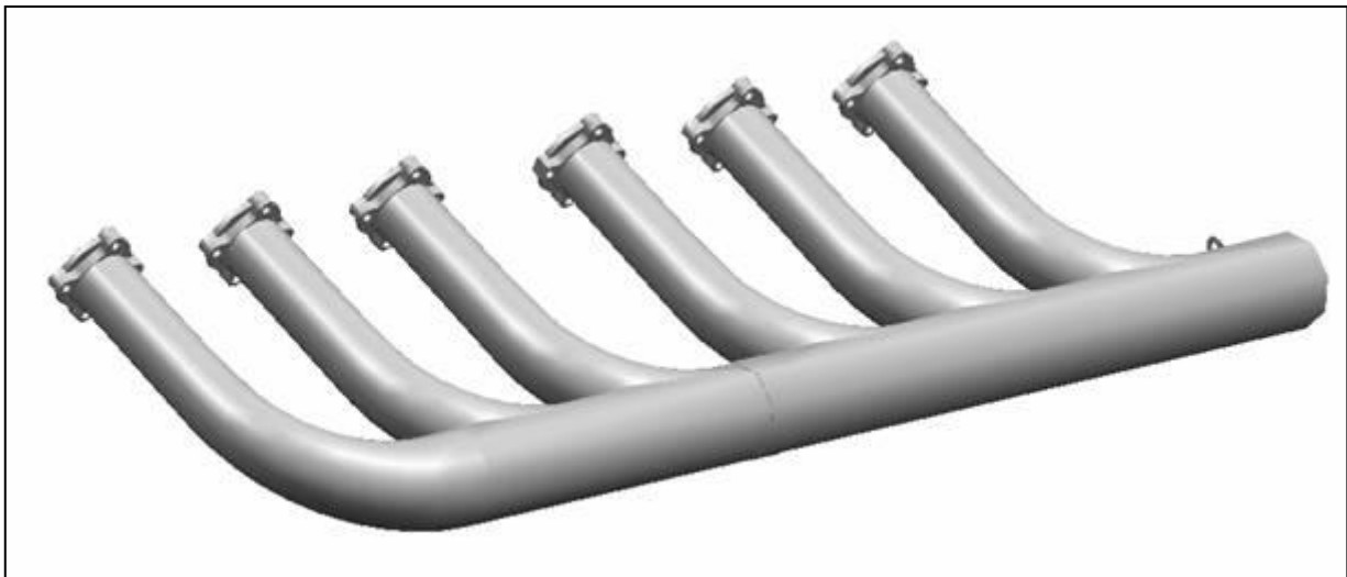
CAD model of the exhaust manifold required to produce the part using Stereo Lithography methods.
