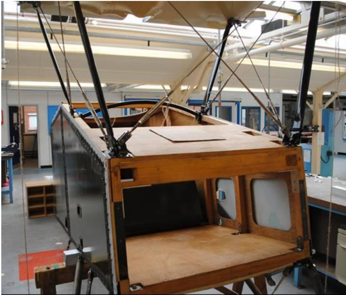
Front end of fuselage with upper centre plane and bracing fitted.
